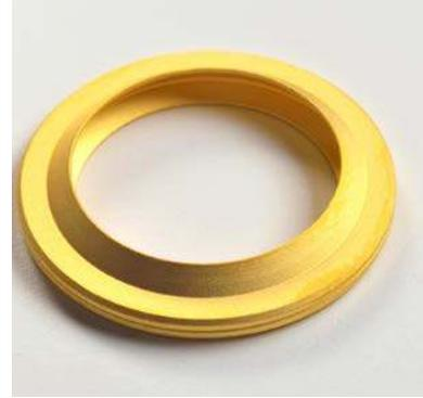
The K-Port seal is designed to prevent fluid leakage and/or pressure loss between a fitting (per AS-933; supercedes MS-33656) and a connection port (per AS-5202; supercedes MS-33649).
