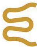
The standard E-FLEX™ design exhibits improved spring back and reduced load compared to C-Rings.
