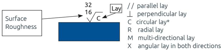
\* Most metal seal applications require a circular or circumferential lay
