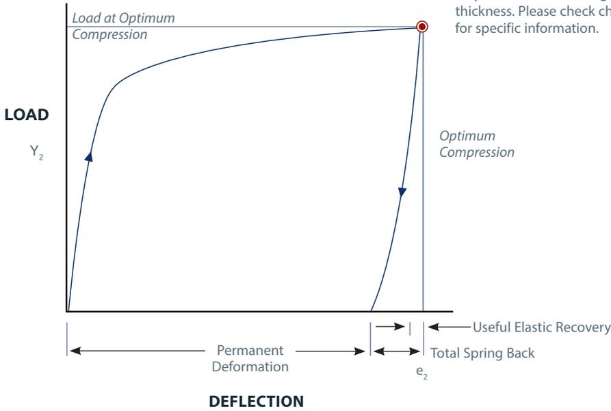
NOTE: Actual spring back and load will vary based on material, geometry, and wall thickness. Please check characteristic chart for specific information.
