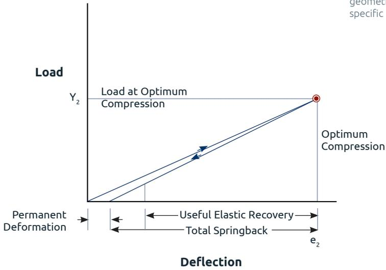
NOTE: Actual spring back and load will vary based on material, geometry, and wall thickness. Please check characteristic chart for specific information.
