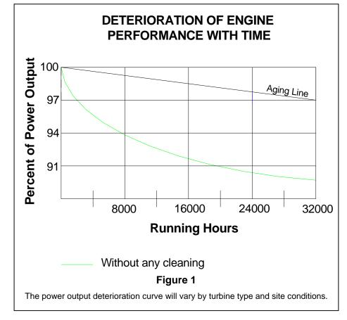
most pronounced in the initial 2000-3000 running hours after an engine has been put into service in a "new clean" and condition. Once contaminants have plated and varnished on the hot airfoil surfaces, the rate of efficiency deterioration decreases and performance tends to stabilize. See Figure 1 for reduction in power output over time. Recovery from the degraded condition is not possible without removing the foulants.
