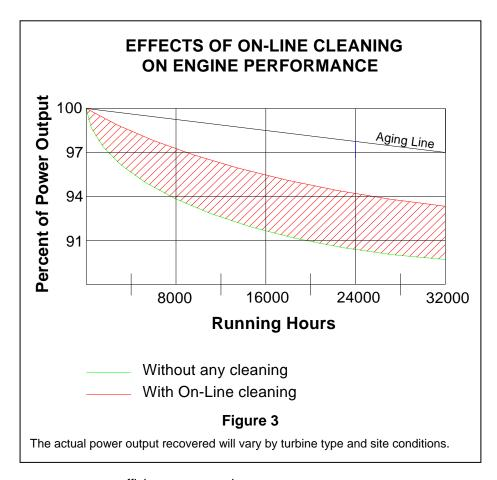
can be maximized. The shaded area in Figure 4 shows that most of the power lost due to fouling can be recovered.
